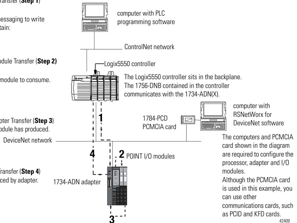
Because the adapter simultaneously resides on the DeviceNet network and on PointBus, it serves as a slave to the processor (i.e., #1 & 4) and a master to the I/O modules (i.e., #2 & 3).
