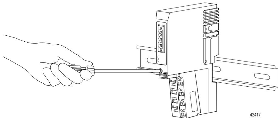
5. Pull the adapter off of the DIN rail to remove it from the existing system.
