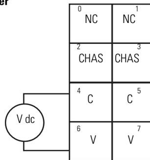
This dc supply is connected to the internal power bus.
